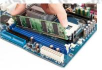
A motherboard is also the main part of a computer because the motherboard is the main circuit of the computer, in which many main parts of the computer are connected such as - RAM, ROM, video card, network card, processor, and power supply.
