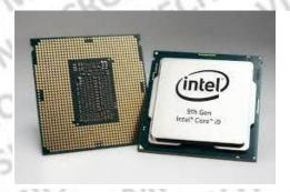
CPU stands for Central Processing Unit. Just like humans have a brain, the CPU is called the brain of a computer. CPU is also known as the processor or Microprocessor.
